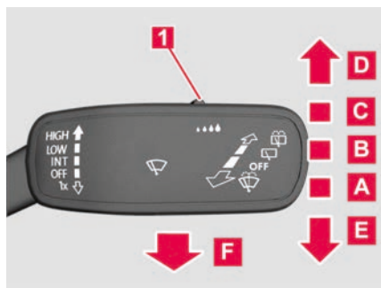
Fig. 66 On the right of the steering column: Operating the front windscreen wipers
