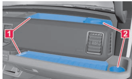
Fig. 121 On driver and front passenger sides: open stowage compartment with drink holder
