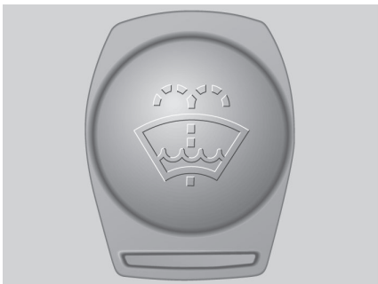
Fig. 188 In the bonnet space: washer fluid reservoir cap.
