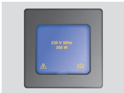
Fig. 127 On the side of the driver seat: 230-volt socket with earthing contact (illustration).
