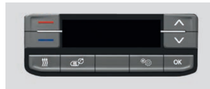
Fig. 74 In the front roof console: Air conditioning block for the rear passenger compartment.
