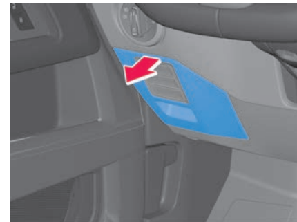
Fig. 176 In the footwell on the driver side: fuse box cover.
