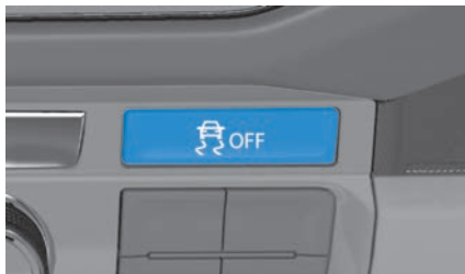
Fig. 120 In the centre console: button for switching TCS on and off manually.
