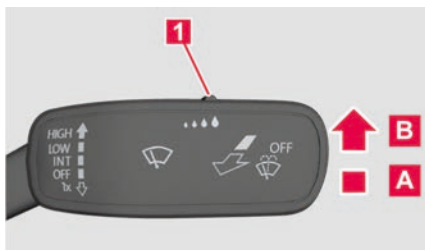
Fig. 68 On the right of the steering column: wiper lever.
