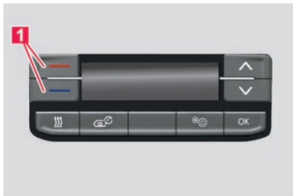
Fig. 75 In the front roof console: Operating the auxiliary heater.
