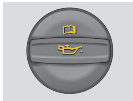
Fig. 192 In the bonnet space: engine oil filler opening cap (illustration).
