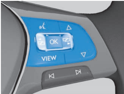
Fig. 15 Right-hand side of the multifunction steering wheel: operating the analogue instrument cluster.
