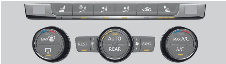
Fig. 72 In the upper part of the centre console: Climatronic air conditioning block.
