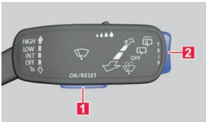
Fig. 16 On the right of the steering column: buttons on the wiper lever.
