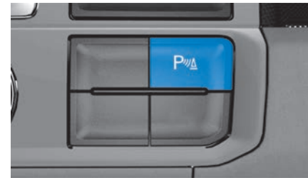
Fig. 106 In the centre console: button for switching the Park Distance Control on or off (with some equipment levels).
