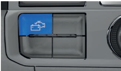
Fig. 130 In the upper part of the centre console: button for maximum battery charge.
