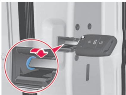
Fig. 44 In the sliding door: Manual locking with the vehicle key.
