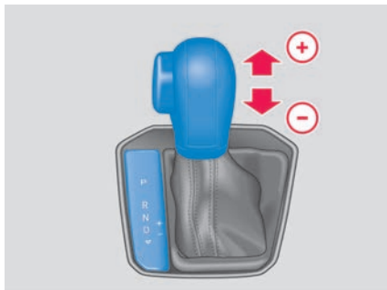
Fig. 83 Selector lever in Tiptronic position (left-hand drive). The controls are mirrored for right-hand drive vehicles.
