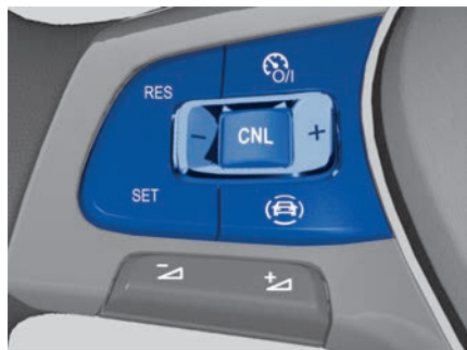
Fig. 99 Left-hand side of the multifunction steering wheel.
