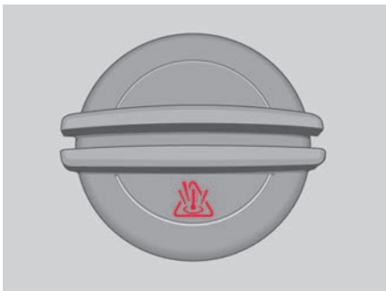
Fig. 193 In the bonnet space: cap of the coolant expansion tank.
