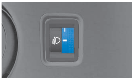
Fig. 65 Beside the steering wheel: slider for headlight range control.
