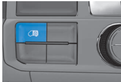
Fig. 47 In the centre console: button for locking the load compartment.
