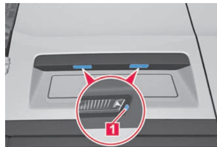
Fig. 170 In the left-hand wing door: Number plate light.
