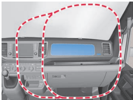
Fig. 31 Location and deployment zone of the front passenger front airbag (illustration).
