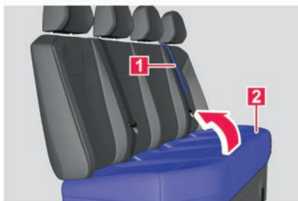
Fig. 59 On the rear bench seat: Fold up the seat cushion.
