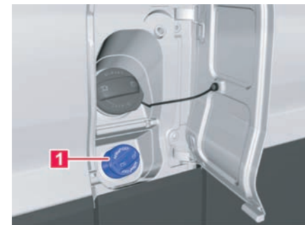
Fig. 153 Behind the tank flap: Cap for the AdBlue filler neck.
