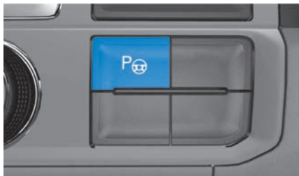
Fig. 111 In the upper part of the centre console: Button for switching on Park Assist.
