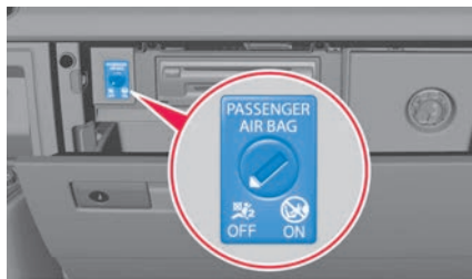
Fig. 32 In the glove box: key-operated switch for switching the front passenger front airbag on and off.
