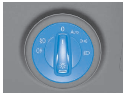
Fig. 63 Beside the steering wheel: light switch (one variant).
