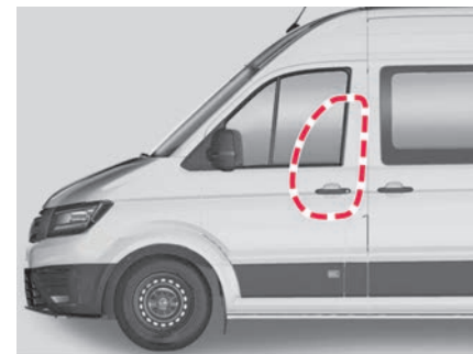
Fig. 35 On the left-hand side of the vehicle: side airbag deployment zone.
