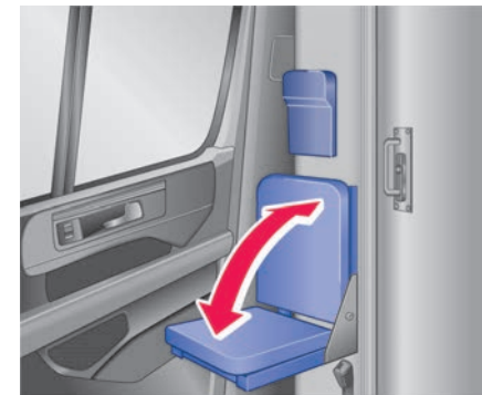
Fig. 58 Next to the load compartment sliding door: folding seat.
