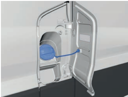
Fig. 151 On the left-hand side of the vehicle: Open tank flap with attached tank cap.
