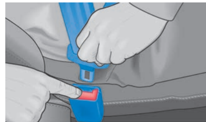
Fig. 26 Removing the latch plate from the buckle
