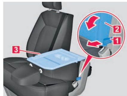
Fig. 124 Front passenger 2-seat bench: folding down the backrest and stowage compartment in the backrest.
