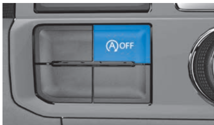
Fig. 86 In the upper part of the centre console: button for the start/stop system.
