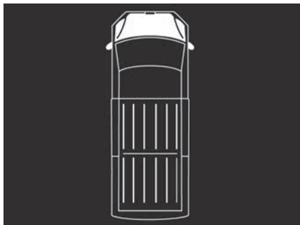
Fig. 187 On the display of the instrument cluster: The bonnet is open or not properly closed (illustration).
