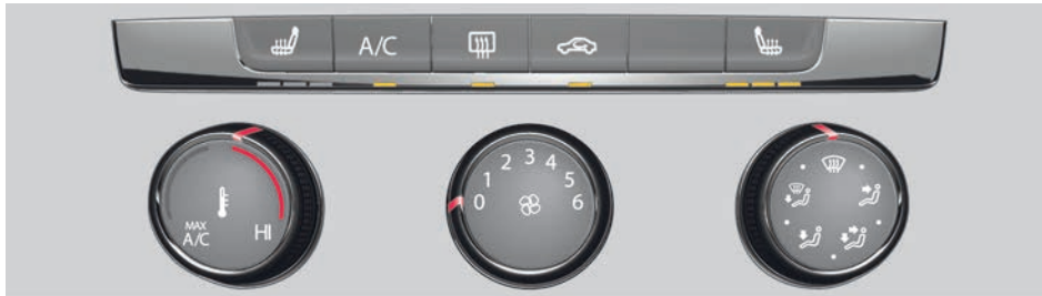
Fig. 73 In the upper part of the centre console: air conditioning block of the manual air conditioning system or the heating and fresh air system.
