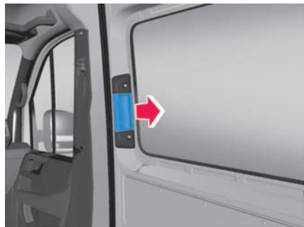
Fig. 43 In the sliding door: Door release lever.
