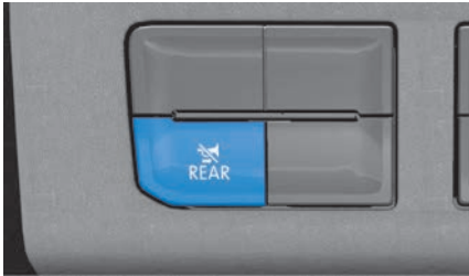
Fig. 107 In the lower part of the centre console: button for the reverse warning system.
