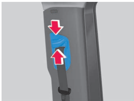
Fig. 29 Next to the front seats: Seat belt height adjuster.
