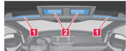
Fig. 122 Under the roof: stowage compartments.
