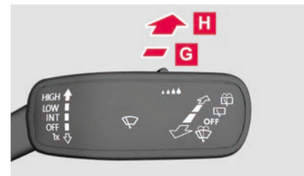
Fig. 67 On the right of the steering column: Operating the rear window wiper.
