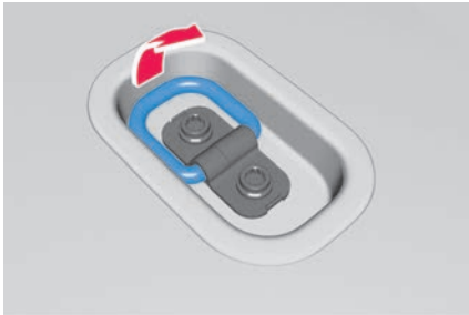
Fig. 137 In the load compartment: fastening rings.
