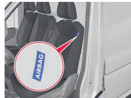
Fig. 36 On the side of the front seat: Location of the side airbag.
