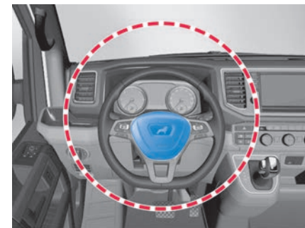
Fig. 30 Location and deployment zone of the driver front airbag (illustration).
