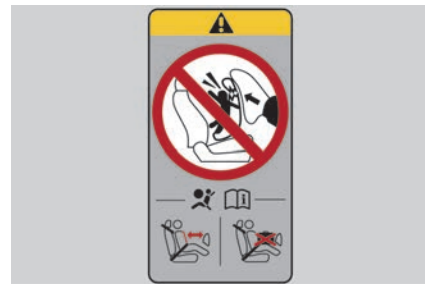
Fig. 40 Diagram: airbag label on the B-pillar.
