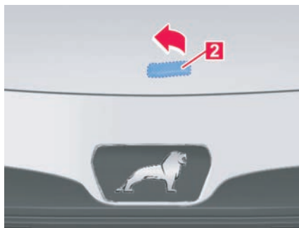
Fig. 184 Above the radiator grille: Lever for opening the bonnet.
